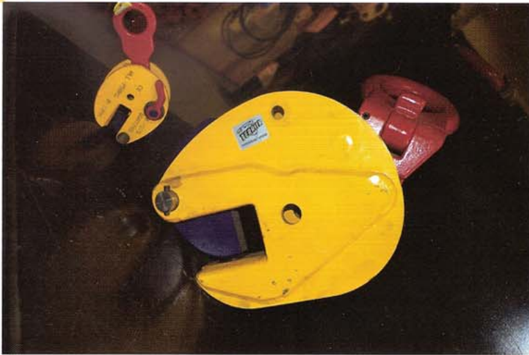
The real thing, lifting clamps clearly marked with all the necessary details to trace it back to the manufacturer
