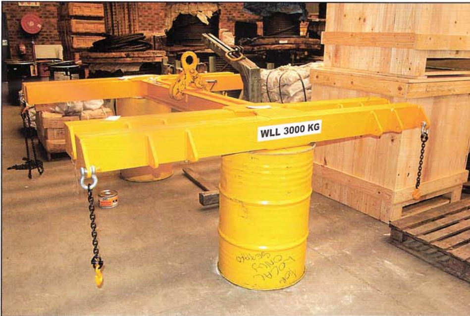
Special lifting equipment has to be designed by an engineer
