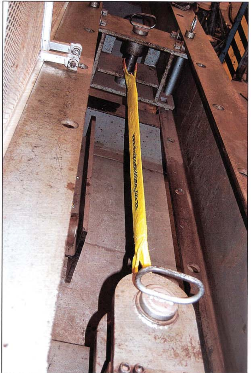
Testing a sling at Elephant's facility
